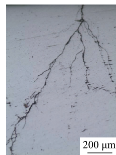
图5 起源于点蚀坑底的裂纹形貌 Fig. 5 Morphology of crack under the pit
