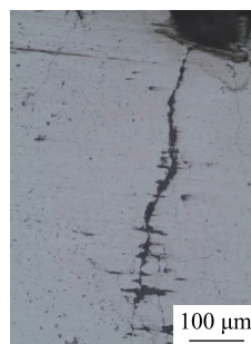
图5 起源于点蚀坑底的裂纹形貌 Fig. 5 Morphology of crack under the pit
